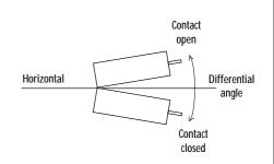
These switches operate when tilted from the horizontal position. The switch movement required to cause contact change (example off to on) is called the differential angle.
