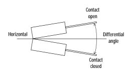
These switches operate when tilted from the horizontal position. The switch movement required to cause contact change (example off to on) is called the differential angle.
