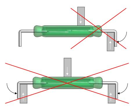
Any form of bending, cutting or modification of the switch leads requires appropriate tooling and fixturing to minimize the introduction of mechanical stress on the glass seal area. Many years of experience has proven that switch damage can be avoided when lead modification is required by proper fixturing and the avoidance of any modification less than 1 mm from the glass seal.
