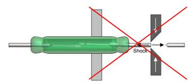
Above demonstrates the creation of a stress component in the direction of the seal, which is the result of clamping the glass body. This is an unacceptable method of modification.
