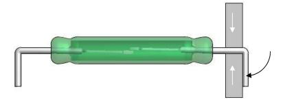
The Figures above and below illustrate bending of the leads. Improper lead bending can be even worse than only cutting. The risk of plastic deformation strain in the NiFe wire leads is very high. Thus, supporting or clamping the lead wire is necessary to avoid damage of the glass seal.
