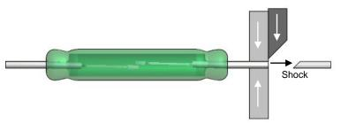
Above an example of a properly clamped lead to avoid improper stresses.
