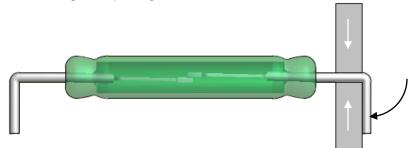
The Figures above and below illustrate bending of the leads. Improper lead bending can be even worse than only cutting. The risk of plastic deformation strain in the NiFe wire leads is very high. Thus, supporting or clamping the lead wire is necessary to avoid damage of the glass seal.
