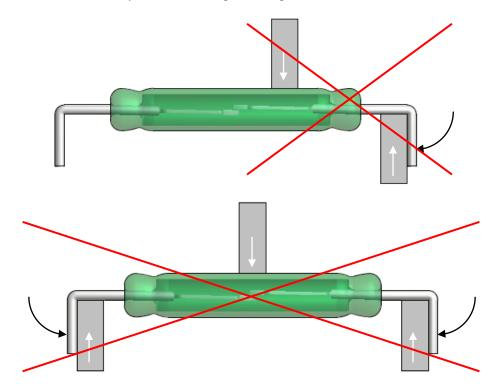
Any form of bending, cutting or modification of the switch leads requires appropriate tooling and fixturing to minimize the introduction of mechanical stress on the glass seal area. Many years of experience has proven that switch damage can be avoided when lead modification is required by proper fixturing and the avoidance of any modification less than 1mm from the glass seal.
