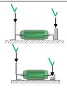
Pressure can be applied directly on the horizontal bended SMD-pad or straight on the vertical bended SMD-pad.
