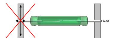
When possible don't add pressure on the glass on placing the reed switch on a pcb or device. However when handling with a Pick and Place machine the acceptable force on the reed switch is 3N with a maximum of 5N
