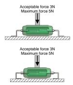
When possible don't add pressure on the glass on placing the SMD switch on a pcb or device. This could result into glass cracks. However when handling with a Pick and Place machine the acceptable force on the reed switch is 3N with a maximum of 5N
