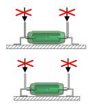
Don't ad pressure on the leads, directly beside the glass-metal connection.
